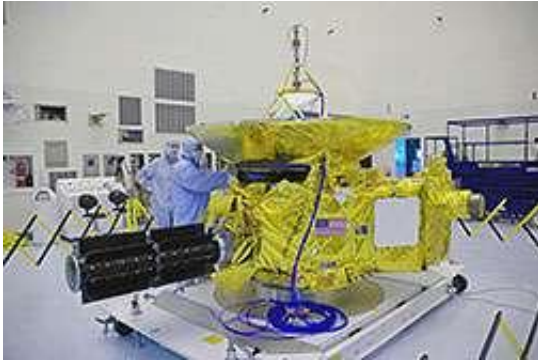
The radioisotope thermoelectric generator (black) undergoing testing during the "hot fit check" in November 2005 prior to the January 2006 launch. Credit: NASA
