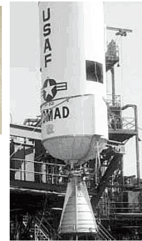
Rocketdyne G-1 LF2/Hydrazine rocket engine for NOMAD Upper Stage System also developed at Santa Susanna
