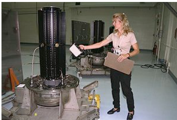
Inspection of Cassini spacecraft RTGs before launch
