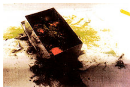
Plutonium pyrophoricity can cause it to look like a glowing ember under certain conditions.
