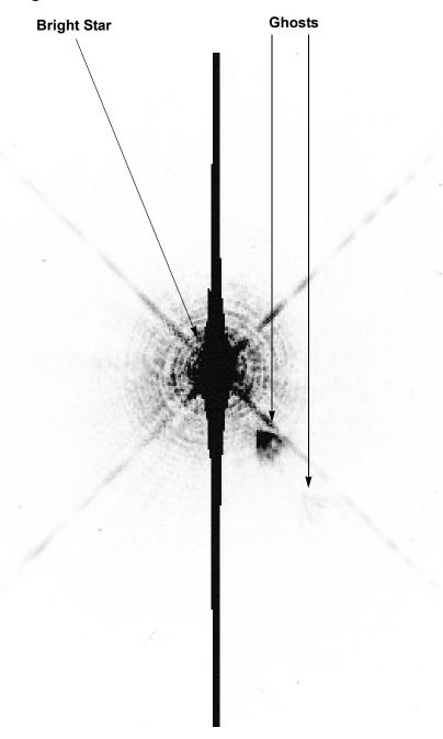
Figure 4.5: Detail of Filter Ghosts on WF4
