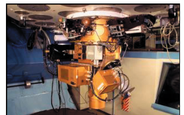
The GoldCam spectrograph, attached to the bottom of the 2.1-meter telescope.
